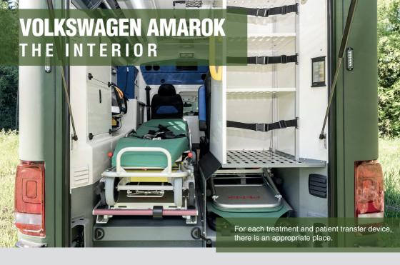
The design of Amarok has been built on the idea of providing paramedics with the best ergonomics and safety as possible. For each treatment and patient transfer device, there is an appropriate place from which they are available quickly and easily. Particular attention is given to safety. All devices are located within arm's reach so that the seat belt does not need to be removed during transport.
