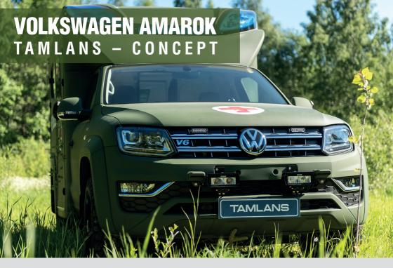
The combination of the chassis with the modular ambulance body is unique. The 190 kW engine power combined with the eight-gear automatic transmission and four-wheel drive gives the opportunity for rapid movement on both asphalt roads and forest trails. The driving characteristics are in a class of their own, even in harsh conditions.
