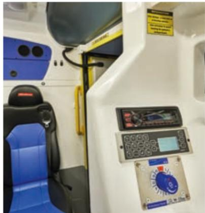
The GDIN control panel is in the patient compartment where it is used to manage a large number of vehicle functions.
