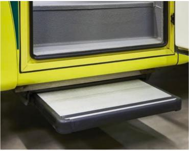
Electrically operated side step at the right front door facilitates access to the patient compartment.
