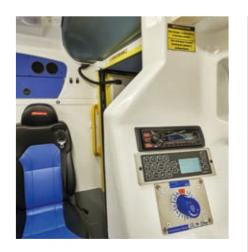
The GDIN control panel is in the patient compartment where it is used to manage a large number of vehicle functions.
