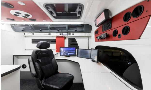
Volkswagen Amarok command centre interior is well designed and easily modifiable work environment. All the equipments and instruments needed are easily found and can be reached while seated in the seat belts. The shelves have illuminated plexiglass windows through which can immediately see what can be found in the shelves. The interior walls are smooth and easy to clean.
