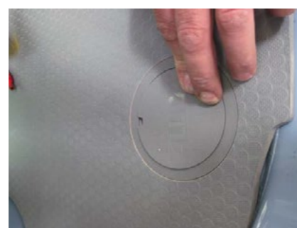
Reattach the lashing point using original screws
