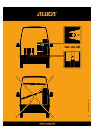
At regular intervals, about every 5,000 km, as well as after an emergency stop or an accident, check the points at which the in-vehicle racking system is attached to the floor and the walls and side connections [rails] and also to lashing points.
